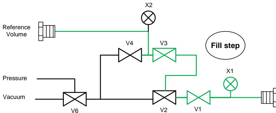
If the pressure in the test chamber meets the tolerance settings, all valves close and trap test pressure in the chamber with the pressure sensor (X1) monitoring the decay.
