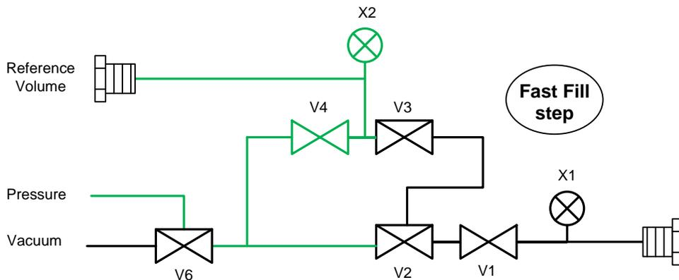
During the **fill** timer, the volume of pressurized air is sent to the test port. This pressure is monitored by (X1). The change in total volume will cause a pressure drop from the initial charge. With a good part in the test chamber, the target pressure will be achieved.
