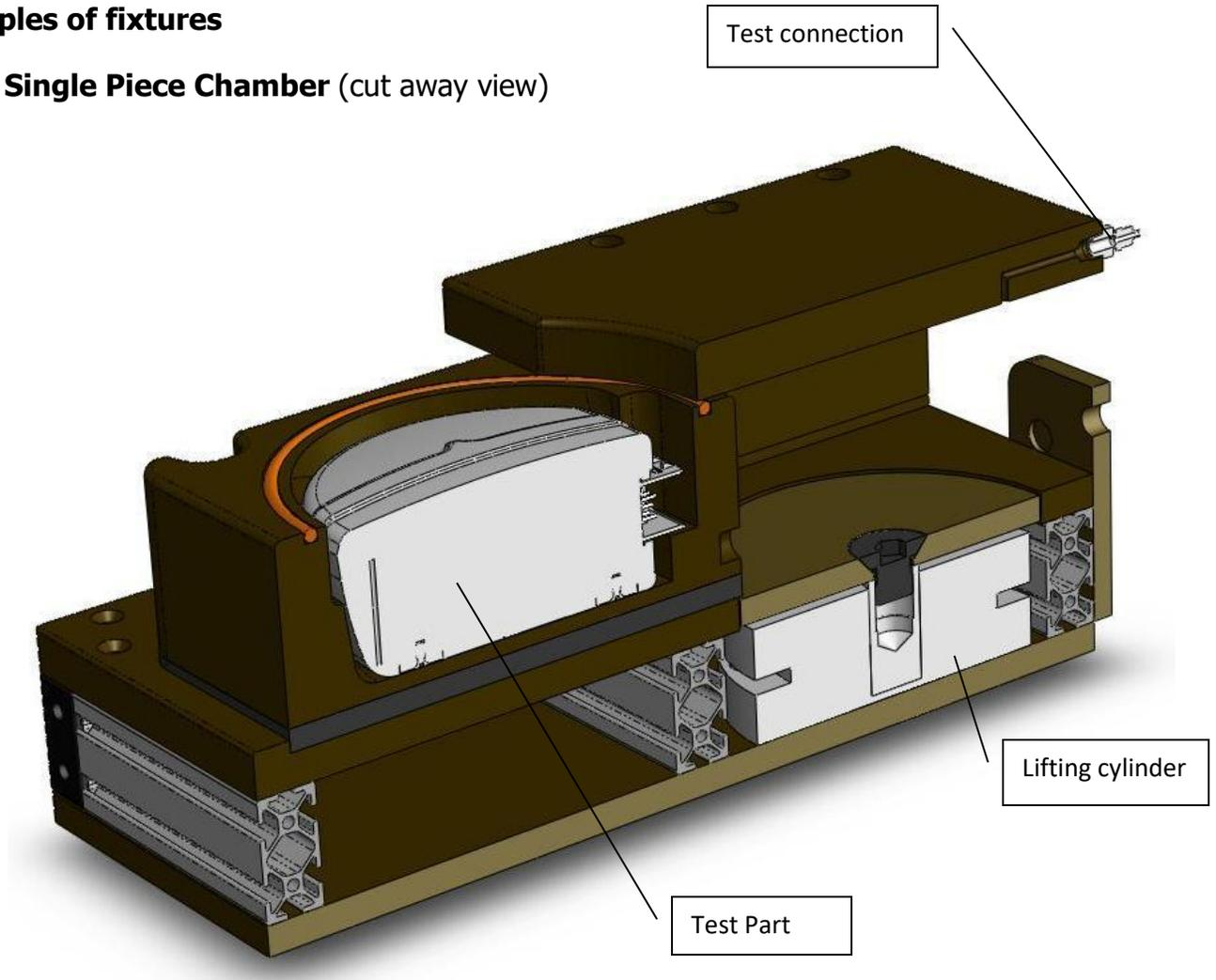
The part is loaded into the nest and slid into the test position. The lifting cylinder seals the test chamber against the top plate.
